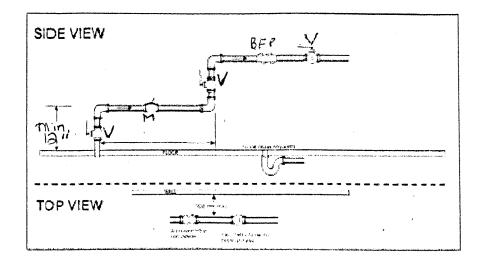
V = Valve M = Meter BFP = Backflow Preventer
